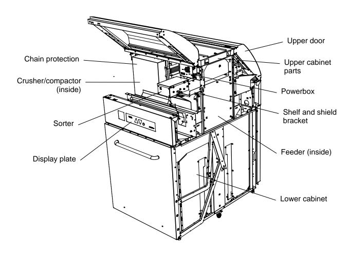
Location of the parts to be disassembled. For detailed description of dismantling procedures, please refer to the *MultiPac Service Manual (70136006)*.
